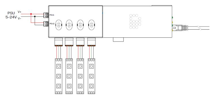
With this setup the Easy Connect can supply a maximum of 30 Ampere to the 4 outputs. PSU1 will supply this to output ports P3 & P4. PSU2 will supply the power for P1 & P2. All output ports will have the same Voltage output.
