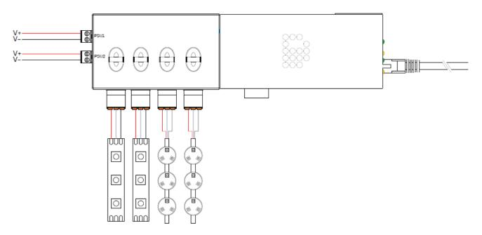
With this setup the Easy Connect can supply a maximum of 15 Ampere for P1 & P2 and P3 & P4. PSU1 will supply this to output ports P3 & P4. PSU2 will supply the power for P1 & P2. In this case the input Voltage of PSU1 and PSU2 can differ. As example PSU1 could be 24 Vdc to power the Modules and PSU2 could be 5 Vdc to power the LED strips.
