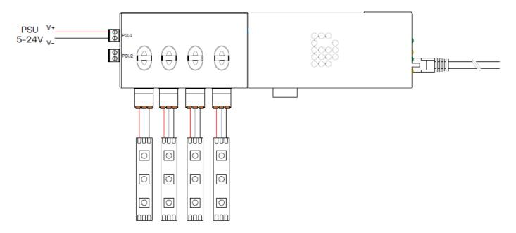
This setup of the Easy Connect can supply a maximum of 15 Ampere to the 4 outputs. All output ports will have the same Voltage output.
