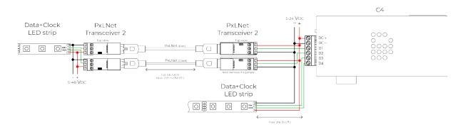
DiGidot Controllers with a PxLNet Transmitter, connected by Cat-5E network cables to PxLNet Transceivers. Please note that DMX TTL must be configured on the DiGidot Controller on the In/out configuration page.
