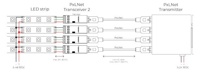
DiGidot Controller with PxLNet Transmitter connected by Cat-5E network cables which are connected to PxLNet Transceivers, which are wired to pixel controlled LED products, that run on another power supply and/or voltage.
