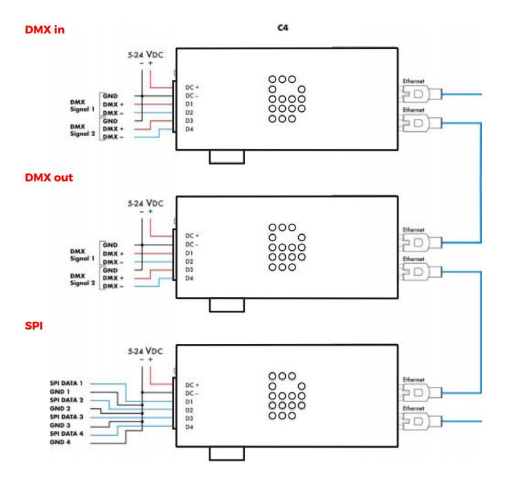
IMPORTANT: All Grounds, from the DiGidot C4 and all power supplies must be connected. The Ground output wires of each Data pair from the DiGidot C4 output must be equal in length as the Data wires.
